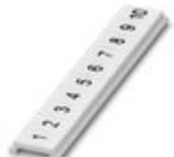
Zack Marker strip, flat, Strip, white, labeled, printed horizontally: consecutive numbers 1 ... 10, 11 ... 20, etc. up to 91 ... 100, mounting type: snap into flat marker groove, for terminal block width: 3.5 mm, lettering field size: 5.15 x 3.5 mm, Number of individual labels: 10
