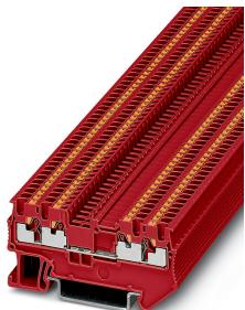
Feed-through terminal block, nom. voltage: 500 V, nominal current: 17.5 A, connection method: Push-in connection, 1 level, Rated cross section: 1.5 mm<sup>2</sup>, cross section: 0.14 mm<sup>2</sup> - 1.5 mm<sup>2</sup>, mounting type: NS 35/7,5, NS 35/15, color: red
